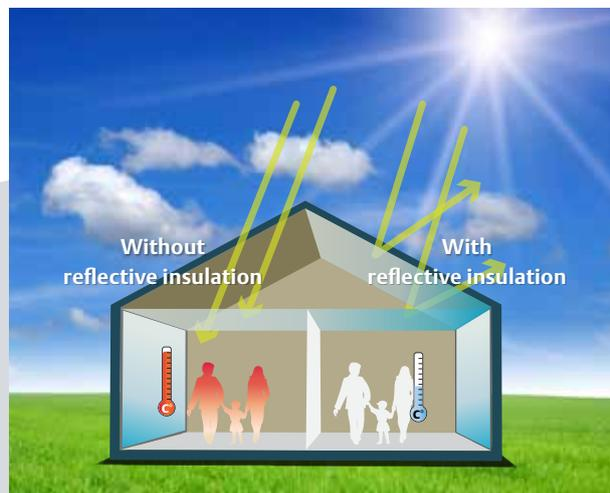
ASTRO-E reflective foil insulation consists of a layer of polyethylene bubble film sandwiched between two layers of 99% pure aluminium foil making the structure 1/4" thick
