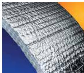
ASTRO-E reflective foil insulation consists of a layer of polyethylene bubble film sandwiched between two layers of 99% pure aluminium foil making the structure 1/4" thick. ASTRO-E saves up to 50% energy.
