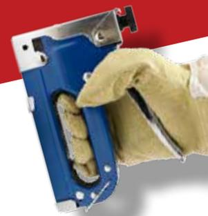
Reflective foil can be cut easily with a razor blade or scissors and installed with common staples, nails or screws.
