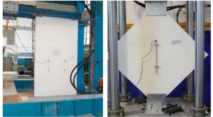
*Shear compression test on a sample portion of panel*
